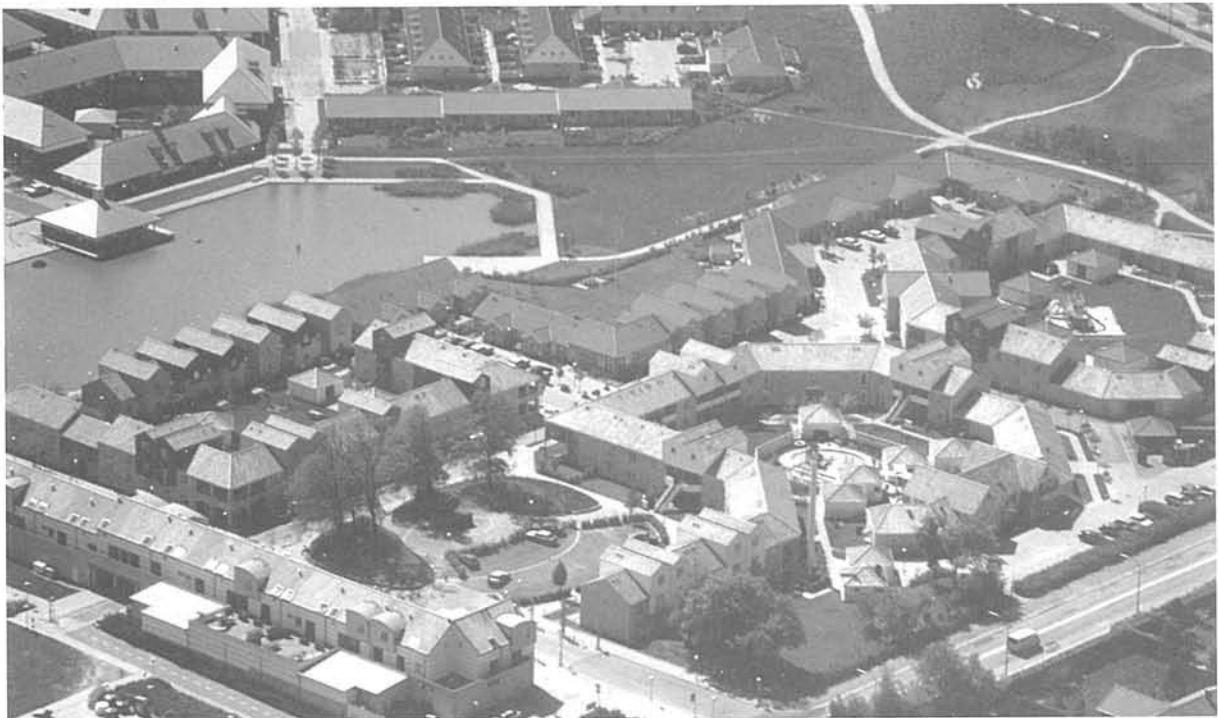
Fig 3. Great emphasis has been placed on the design of the urban space. An urban form with a varied environment has been achieved. Buildings are joined to their neighbours and placed directly on the edges of streets. Pavements and plantation contribute in forming a sense of a town unit.
