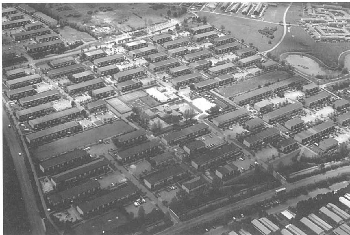
Fig 5. The linear building scheme is demonstrated on the photo. The pathways do not support the creation of a housing area with vitality. That is in the sense that they form a rigid pattern and the pathway's only purpose is to give access to the houses. In a crime preventional perspective it is less favourable because of the many entrances to the area, its monotonous enclosure and the lack of visibility.
