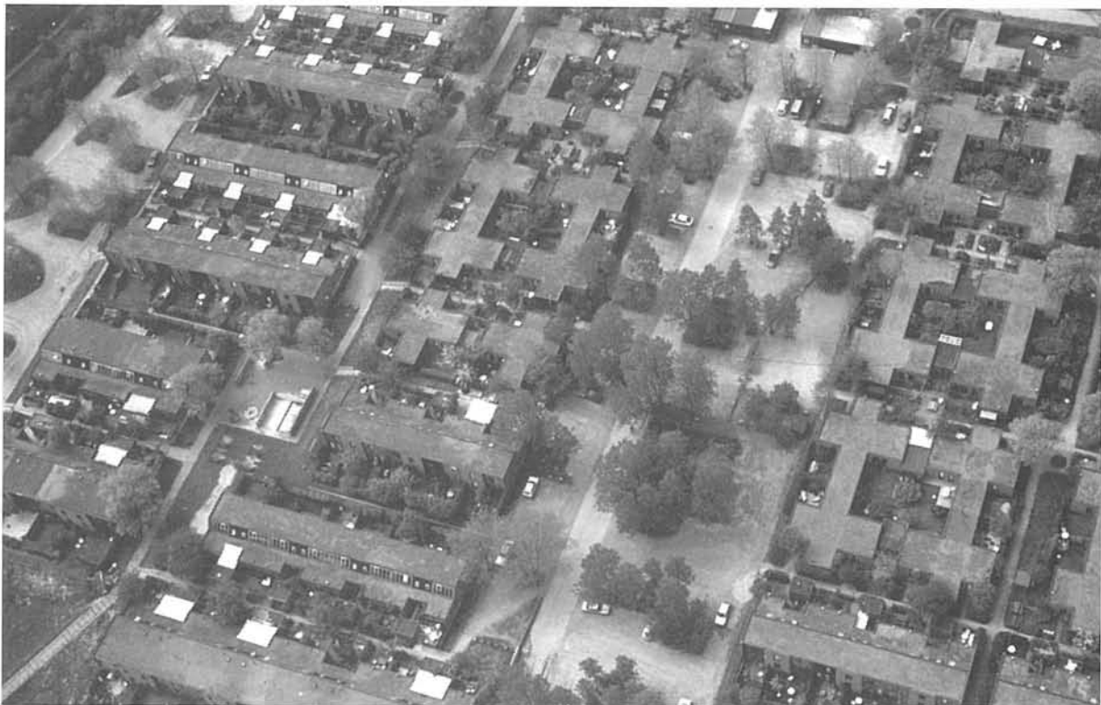
Fig 4. Galgebakken's "step up" system is clearly visible on the air-photo with the semi-detached houses forming the housing quarters. The traffic system can also be detected with the pathways for pedestrians and the parking places in between as pockets with only one way in and out.
