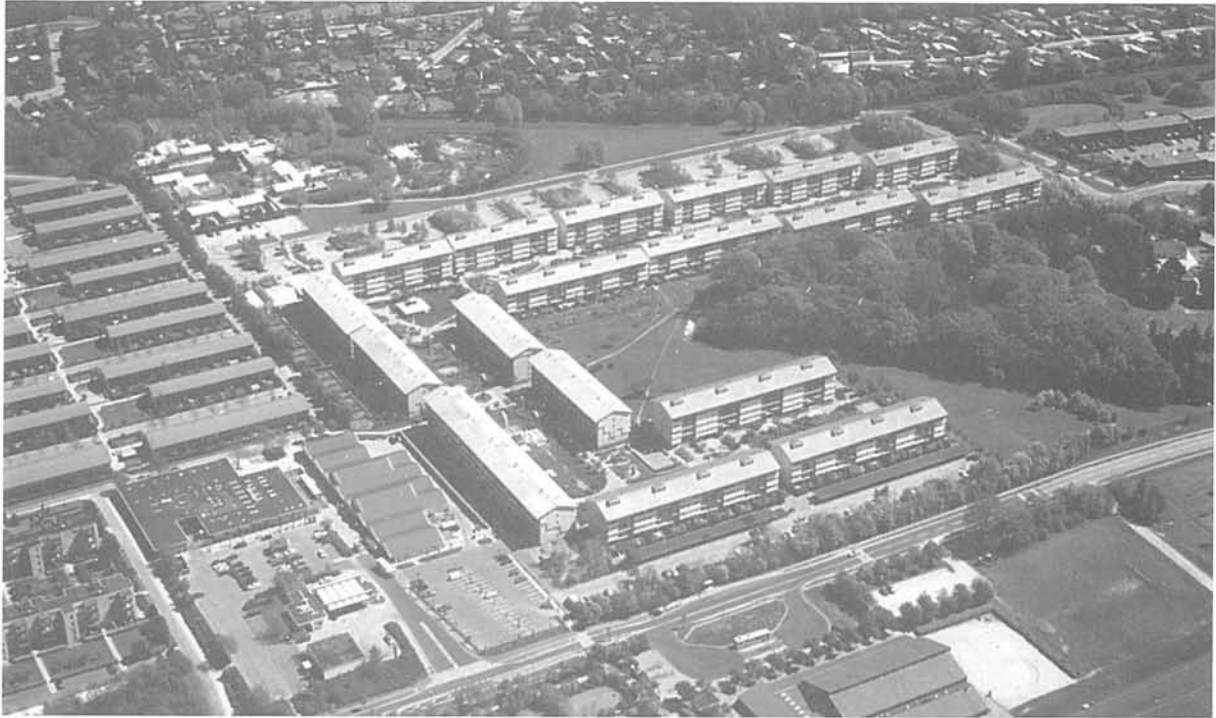
Fig 6. Egedalsvænge, built in 1973 and renovated in 1986, comprises eighteen four-storey blocks of flats with a total of 496 dwellings, 166 minor dwellings for single young people and eight institutions. The inner part of the housing area is car-free, entrances are from inside the common area with playgrounds and open spaces. The parking places are located in the periphery.
